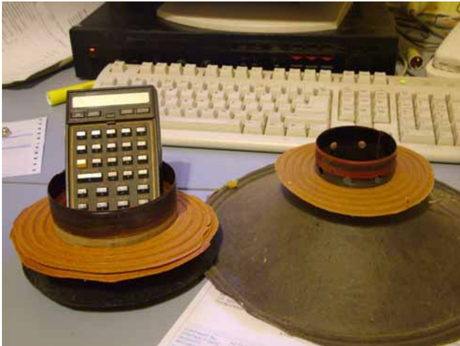
Photograph 2 Comparison of 70 Watt and 20 Watt HF drivers The 70 Watt magnet assembly is under the LHS of the calculator and the Voice coil assembly under the RHS
