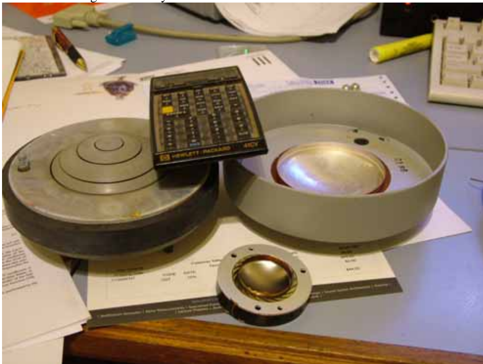
Photograph 2 Comparison of 70 Watt and 20 Watt HF drivers The 70 Watt magnet assembly is under the LHS of the calculator and the Voice coil assembly under the RHS
